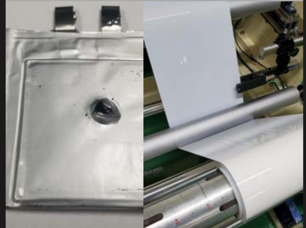
NPORE ® separator prevents thermal runaway in a nail penetration test
